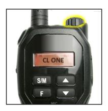
To Resume Normal Usage Turn all of the radios off and back on to resume normal usage after cloning is complete.
