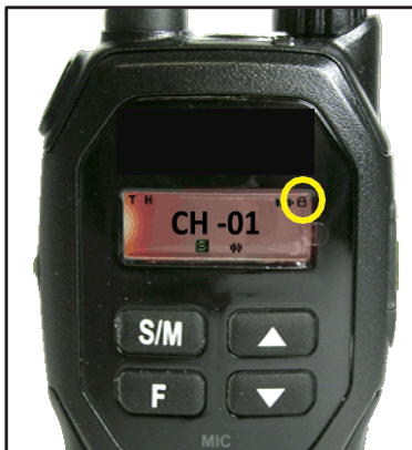
How to Know it's Working The radio will beep and a lock will appear in the upper right corner of the screen.
