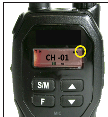
While Locked The Push-to-Talk and F button will still work. The S/M and arrow keys will not.
