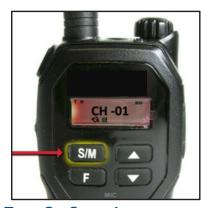
**Turn On Scanning**Press the key programmed as "Scan," a short press of the S/M is the default.
